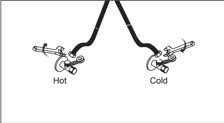
Proceed to connect water lines onto the respective water valves (we recommend using plumbers tape to prevent leakage). Once you've connected the water lines, turn on the water valves.
