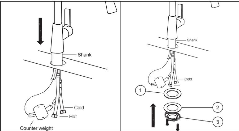
Connect hot and cold flexible hoses to the faucet. Install the faucet through the deck mounting hole. Be sure to align the faucet in the direction desired. Install the rubber washer (1), metal washer (2) and metal base clamp (3). Make sure the plastic base is installed with the flat side facing the deck. Reinstall hose connector if it was removed during installation.
