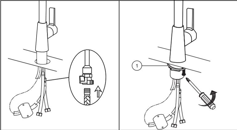
Push the pull-out hose into the hose connector until you hear a click. Use the provided screws by screwing them into the metal base clamp (1). Screw them tightly without stripping the screw heads to secure the faucet.
