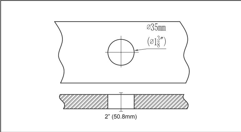
The deck hole should be 1 3/8" (35mm) and the deck thickness should be no more than 2" (50.8mm).
