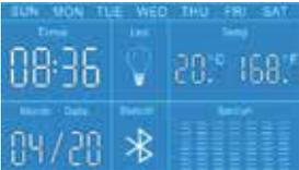
First, power on the unit, Bluetooth symbol will begin to blink. Use your phone/tablet to search for the Bluetooth name "smart mirror". Speaker will play notification sound once connected. Meanwhile, the Bluetooth symbol will stop blinking.
